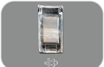
Diesel Particulate Filter (DPF) Switch Regeneration Switch on the dashboard
