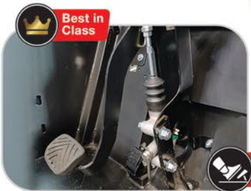
Hydro Pneumatic Clutch 51% reduction in operating effort to significantly reduce operator fatigue
