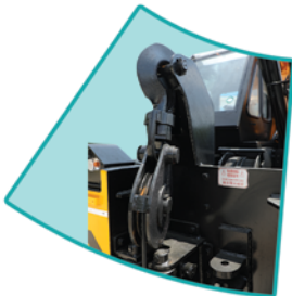
5 t Load Pull* Drag winch for horizontal pulling or dragging of load
