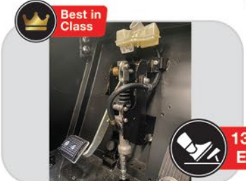
Hydro Pneumatic Clutch 51% reduction in operating effort to significantly reduce operator fatigue
