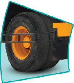
Tyres 11 x 20 - 16 PR Industrial grade same size tire helps interchangeability with each other with wheel guard
