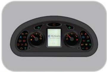
Digital Display Bright and easy-to-read, Single digital cluster with all gauges, fault code detection for engine system. Regeneration text pop-up flashed on display for operator convenience & actions
