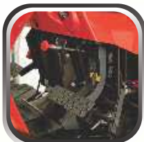
Suspended pedals improves operator's comfort
