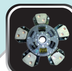
5 Fin cerametallic double clutch 25% more durability
