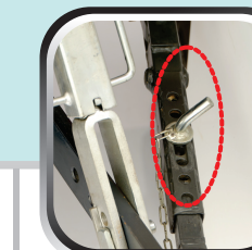
Telescopic stabilizer for easy setting
