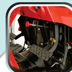
Suspended pedals improves operator's comfort
