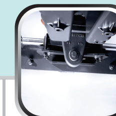
Double acting power steering with variable front axle
