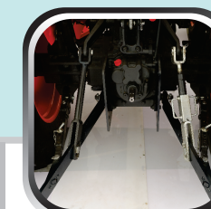
High hydraulic lift capacity 1,800 kgf and 2,100 kgf (at lift point)
